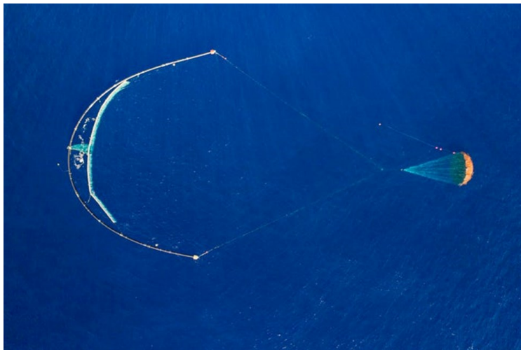
OceanCleanup's passive device to capture floating plastic in the ocean. From: https://theoceancleanup.com .
